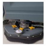
two step:Put the brush cover with a brush bracket and use a plastic knob to tighten.
