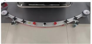
4.4.3 Unscrew the nut of the water suction lever component, remove the bottom plate of the water suction lever component, and remove the front and rear rubber strips of the water suction lever
