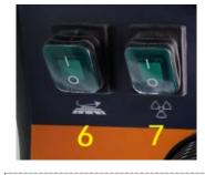
three step: Open the panel work buttons 6 and 7, and the brush and suction cup will automatically fall down. Press the accelerator pedal to start working.
