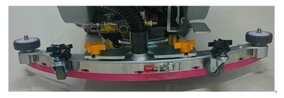
3.2.1.2 Adjust the water volume to the appropriate position through the water valve switch under the machine head(It depends on the dryness of the ground. The machine must be operated with water brushes. Sufficient water should be maintained during the operation. Do not dry-suction to prevent dust from entering the suction motor and causing the suction motor to malfunction)
